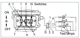
Fig. 8 Connection of the test lamps
