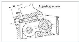
Fig. 7 Dimension a for the adjustment of the adjusting screw
