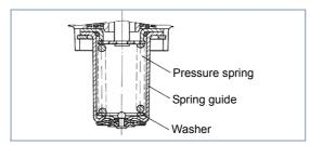
Fig. 8 Position of the washer
