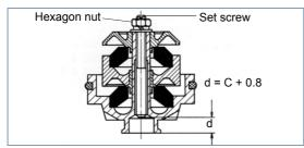
Fig. 5 Dimension d (Device with two rubber springs)
