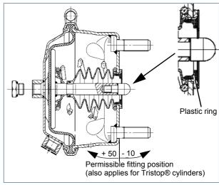
Figure: Cross-section of the membrane cylinder
