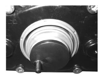
Install the pressure plate and the brake linings, and set the clearance, see chapter "7.4 Fitting the brake linings" on page 29.
