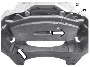
The pressure plate must always be placed correctly in the guide groove (arrow) of the brake anchor plate and is to cover the entire surface of the guide strips of the brake anchor plate. Otherwise the pressure plate could slide out of the guiding.
