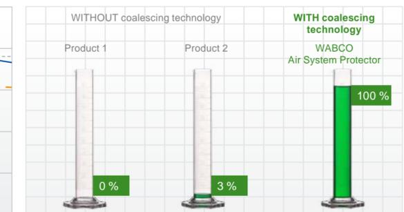
Test conditions: 704 cm<sup>3</sup>-two-cylinder-compressor at high temperature setting, 12.5 bar and 50% duty cycle; calculation based on aerosol measurement downstream the air-dryer
