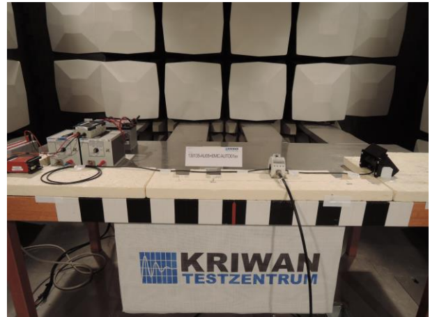
Figure 6: A.RI - BCI - 450 mm from EUT
