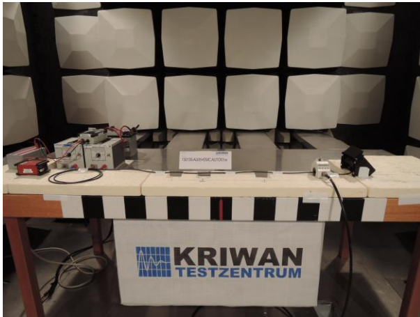
Figure 5: A.RI - BCI - 150 mm from EUT
