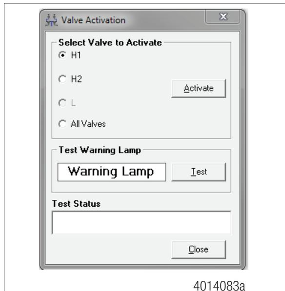
2. The H1 valve indicator will be selected. Click on the **Activate** button and listen for the valve to click, indicating a good installation. The Test Status box at the bottom of the menu will also display the status of this test.
