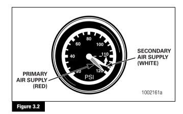
When the compressor is in the **loaded cycle**, air pressure will build to approximately 120-140 psi (827-965 kPa) (cut-out pressure). When the compressor reaches the **unloaded cycle**, the air dryer will purge, initiating regeneration of the air dryer.
