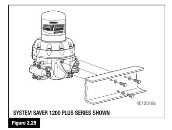
4. Attach the new unit to the frame or mounting bracket with new mounting capscrews and washers. Tighten the capscrews to 22-30 ft-lb (30-40 №m). Figure 2.26 and Figure 2.27.
