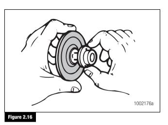
10. Install spring in valve head; fit valve head assembly into bore.
