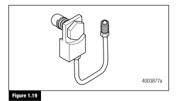
**ECON Valve:** This valve must be installed if System Saver 1200 Series air dryers NOT DESIGNATED E are used with Holset E-type compressors. This valve is not required on System Saver 1200 E air dryers. Figure 1.20.
