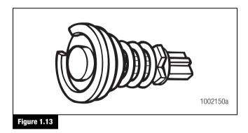
**Outlet Check Valve:** A valve located in the outlet port (port 21) of the air dryer. It prevents air from flowing back through the air dryer and escaping out the purge valve during a compressor unload cycle. Figure 1.14.
