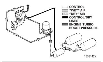
Compressed air passes into the air dryer at the inlet port:
