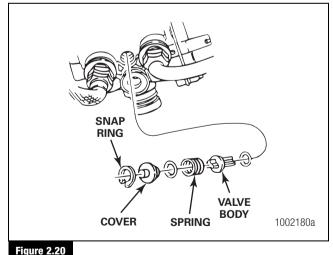
7. Install the new spring so it fits around the "Y"-shaped fins on the valve body.
