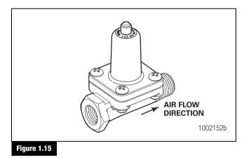
**Pressure Relief Valve:** A valve that protects the air dryer from over-pressurization. On dryers with date codes earlier than 2295, it is installed in the inlet port of the dryer (port 1) using a Street-Tee fitting. On dryers with date codes later than 2295, the pressure relief valve is attached directly to the air dryer. Figure 1.16.
