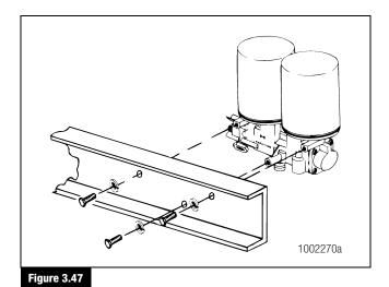
4. Attach the new unit to the frame or to the mounting bracket with new mounting capscrews and washers. Tighten the capscrews to 22-30 lb-ft (30-40 N•m). Figure 3.48. ①
