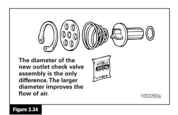
Remove the snap ring from System Saver Twin air dryer Port 2.
