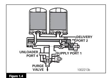
At 60 psi (413 kPa) or greater, the System Saver Twin air dryer switches air flow from the other cartridge every 60 seconds.
