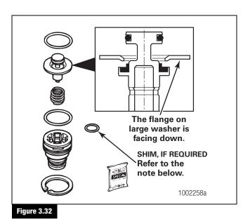
**NOTE:** The shim may not be included with the kit. If it is not included, it is not required. If it is included, install it between the spring and valve head.
