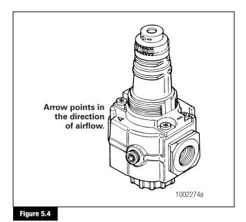
The back-pressure control valve maintains adequate pressure at the outlet of the System Saver Twin air dryer to ensure correct operation in high air usage applications.
