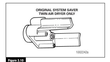
**NOTE:** The right piston cover houses the solenoid/armature and charging valve assemblies. Carefully remove and save these assemblies. Clean and inspect them before reinstalling them in the new cover. You must also remove the right piston assembly when replacing the cover.
