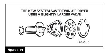
**Purge Valve:** Allows the collected moisture and contaminants to be expelled from the System Saver Twin air dryer during the unloaded cycle. The purge valve remains open for the entire compressor unload cycle. Figure 1.15.
