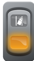
Fault Condition GREEN OFF/AMBER ON (Refer to Flashing Code Operation)
