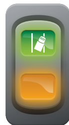
Not Ready to Assist GREEN ON/AMBER ON
