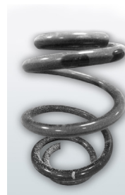
WABCO's parking spring after corrosive slurry/mud test*
