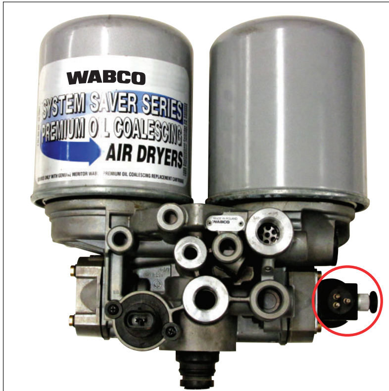
Twin Chamber Air Dryer with Indicated Timer Element
