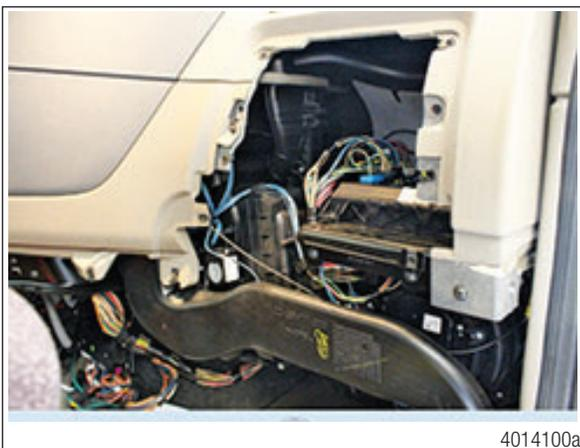
2. Starting at the B-panel location, feed the A leg of the cab harness in the direction of the instrument cluster and down to the left side kick panel area. Feed the B leg of the harness toward the engine bulkhead connector. Feed the C leg of the harness toward the cab bulkhead connector. Leave the D leg of the harness at the B-panel opening. Feed the E leg of the harness toward the SAM cab in the glove box area.
