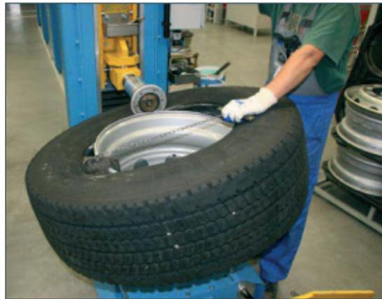
5. Remove the complete wheel from the assembly machine.
