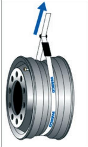
4. Tighten the fastening strap with a tensile force of ~100 Nm and close the Velcro fastener.
