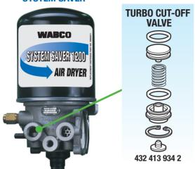
System Saver U Series, UP Series, and 1800UP Series have no spring in the turbo cut-off valve. When using repair kit (R950013) for those models, discard the spring.
